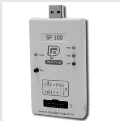
Figure 19-8: A Dediprogram SF100 ISP IC Programmer
