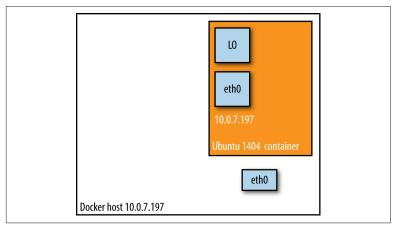
Figure 2-3. Docker host mode networking setup
