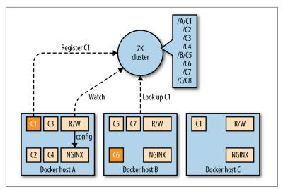
Figure 4-1. Example service discovery with ZooKeeper
