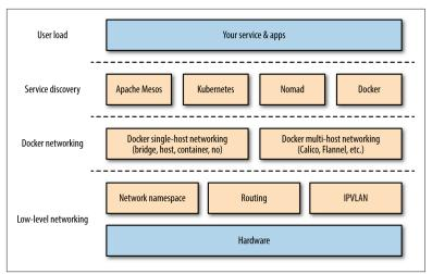
Figure 1-1. Docker networking and service discovery (DNSD) stack
