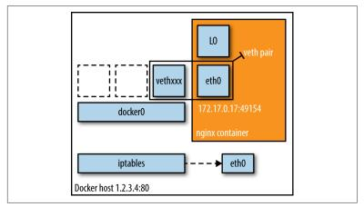
Figure 2-2. Bridge mode networking setup
