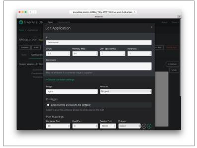
Figure 5-8. The Apache Mesos framework Marathon, launching an NGINX Docker image
