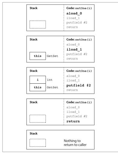
Figure 3-2. The JVM stack for setOne()
