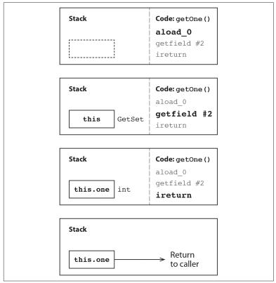
Figure 3-1. The JVM stack for getOne()
