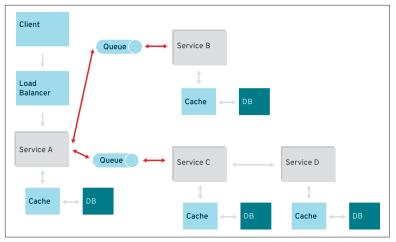
Figure 5-5. Asynchronous messaging
