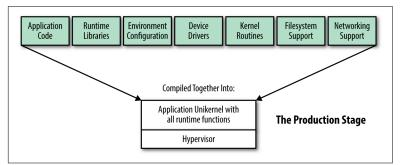
Figure 2-5. Unikernel deployment stack
