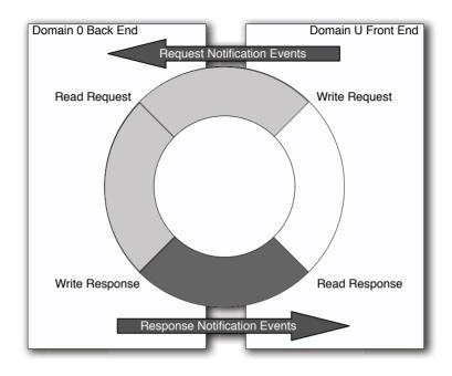
Figure 6.1: The composition of a split device driver
