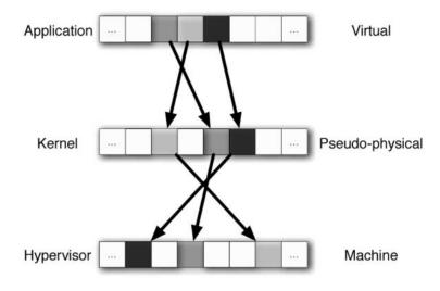
Figure 5.1: The three layers of Xen memory
