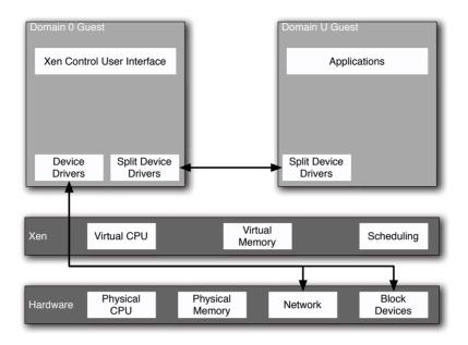
Figure 1.6: A simple Xen configuration
