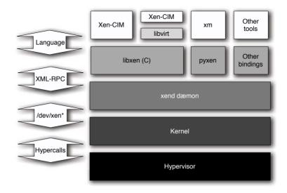
Figure 11.1: The Xen interface hierarchy
