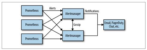
Figure 20-2. Clustering architecture for the Alertmanager
