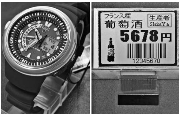
Figure 6.54 (a) Citizen watch (U-100) with FLC display and (b) prototype panel for electrical label system [69].
