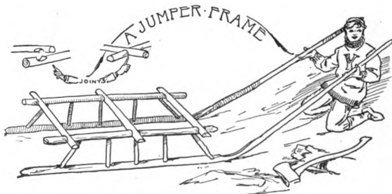
Fig. 465.—Notice that the shafts are cut thinner near front of runners so that they may bend at these points.
