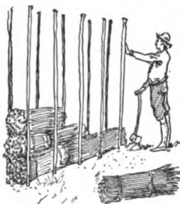
Fig. 212.—Lay up the brush as you would a stone wall.
