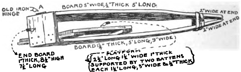
Fig. 41.—A log cabin press used at the author's camp, made of material from the rubbish heap.
