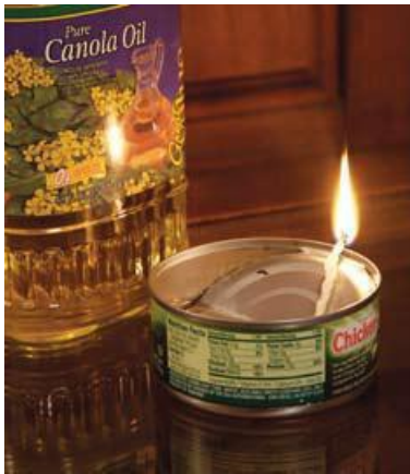
7 Homemade oil lamp made from a tuna can, cooking oil, and a wick created from a strip of paper towel.
