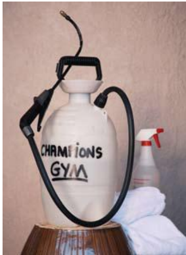
B.O. busters. Both the large pressurized sprayer and the hand spray bottle can be painted black or a dark color for better heat absorption from the sun.
