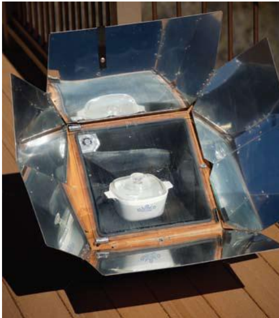
Pasteurizing nonpotable water in a commercial solar oven.
