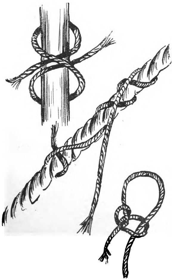
THE CLOVE HITCH ; THE ROLLING HITCH ; THE RUNNING BOW-LINE
