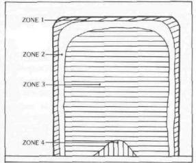
Figure 89 Temperature zonation during Short Composting.
