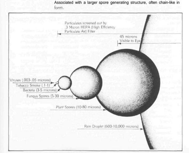
Figure 177 Diagram illustrating comparative sizes of airborne particulates.
