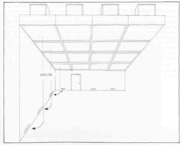
Figure 241 Sterile room with ceiling composed of micron filters.
