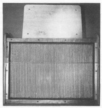
Figure 240 A commercially available laminar flow hood.
