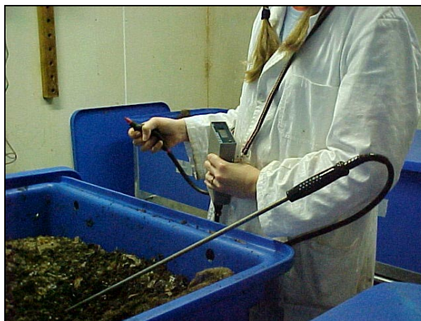
Plate 1. Monitoring temperature and oxygen within a vermiculture unit. Management and maintenance will enable a vermiculture unit to operate effectively.
