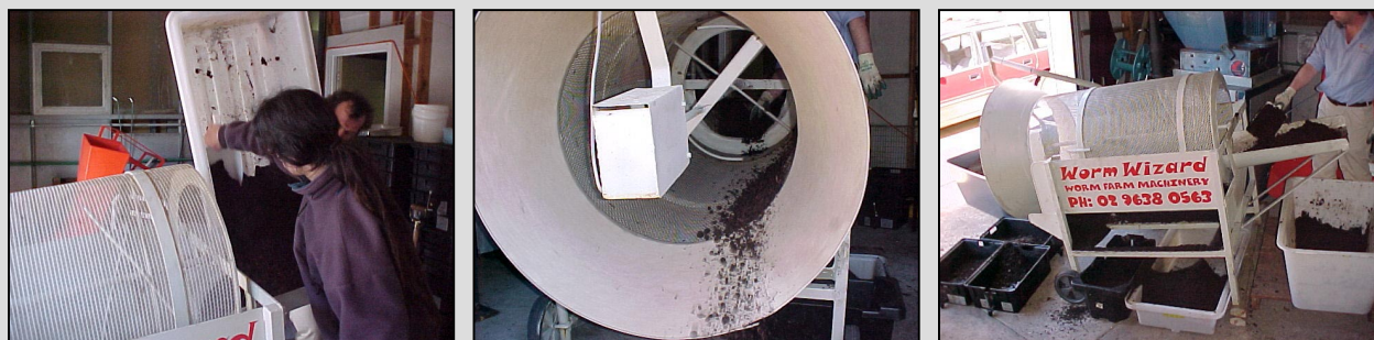
Plate 3. Separation of worms and vermicast using a trommel screen to determine the worm biomass at the completion of the trial. The worms and vermicast are fed into the trommel screen (left) which rotates (centre) and separates the worms from the vermicast (right).
