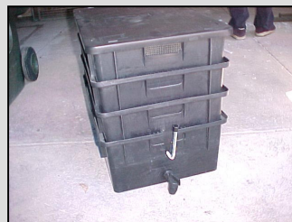
Plate 2. Bench-scale vermiculture units used in the trial (left) showing the perforated bottom and sliding mechanism (right).
