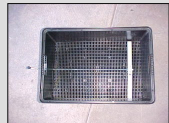
Plate 2. Bench-scale vermiculture units used in the trial (left) showing the perforated bottom and sliding mechanism (right).
