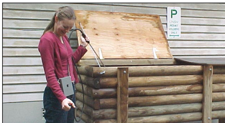
Plate 14. Insert oxygen probe into the desired zone and aspirate the bulb until the reading becomes steady.
