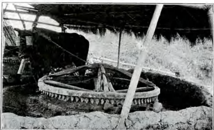
Fig. 158—Close view of power wheel with cow attached, used in driving the irrigation pump, one of the two seen in Fig. 157.
