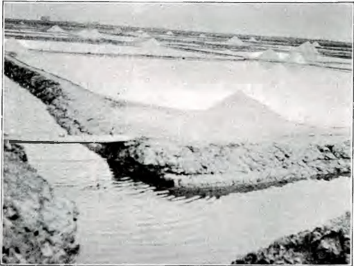
Fig. 197.—Near view of evaporating basins with piles of salt ready to be removed from the fields.
