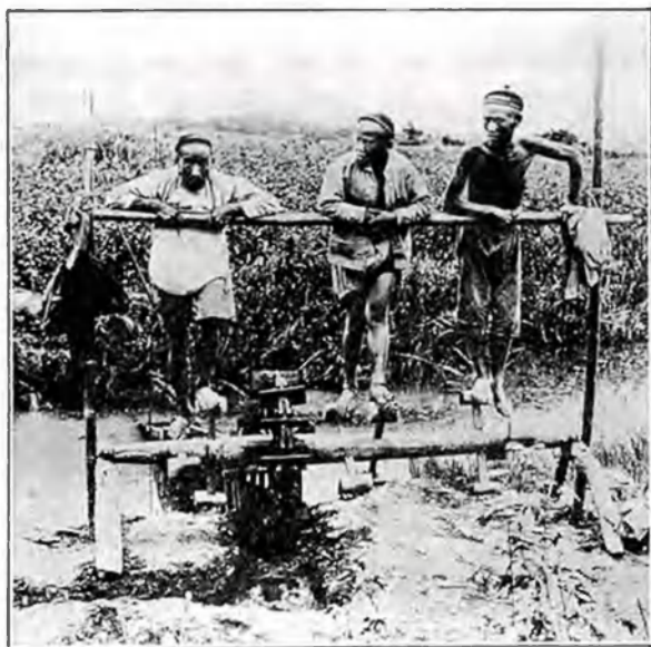
Fig. 42.—The wooden foot-power of China, being used to propel the wooden-chain irrigation pump.
