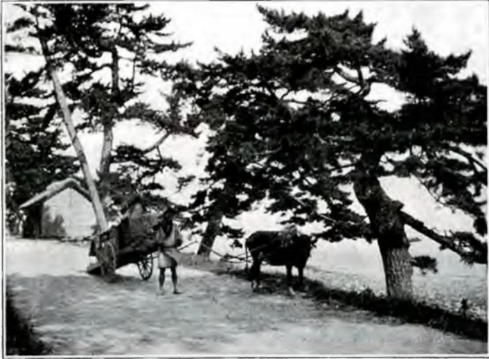
Fig. 108.—Type of conveyance extensively used in Japan for the removal of city and village waste. Such carts are even more frequently drawn by men than by cattle or horses, and tightly covered casks supported on saddles are borne on the backs of both cattle and horses, while men carry pails long distances on their shoulders, using the carrying pole.
