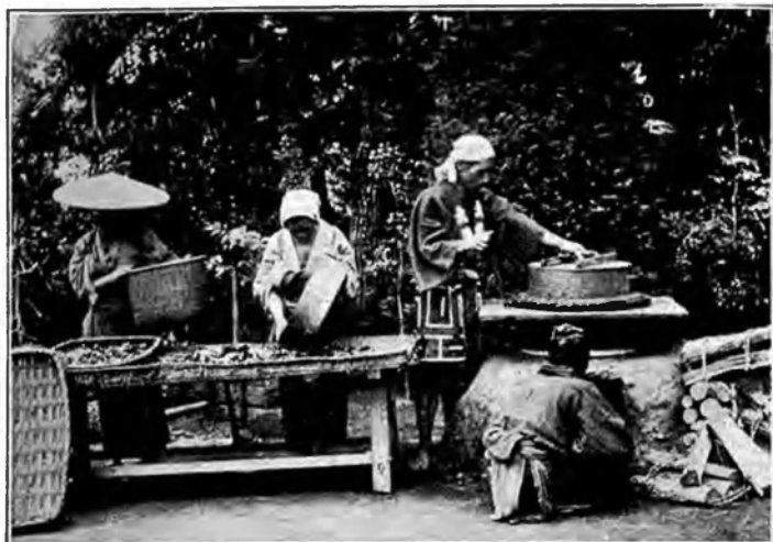
Fig. 77.—Appliance for steaming tea leaves, used in Japan and the same in principle as used in China for steaming meal from which oil is to be expressed.
