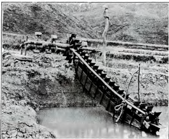
Fig. 171.—Three-man Chinese foot-power and wooden chain pump extensively used for irrigation in various parts of China.
