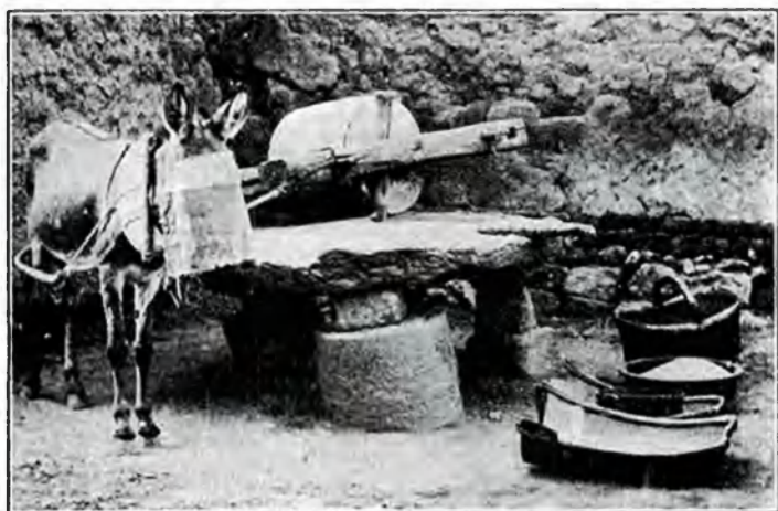
Fig. 64.—Stone mill in common use for grinding beans and various kinds of grain.
