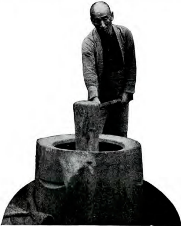
Fig. 179.—Large wooden mortar used for the polishing of rice in Japan.
