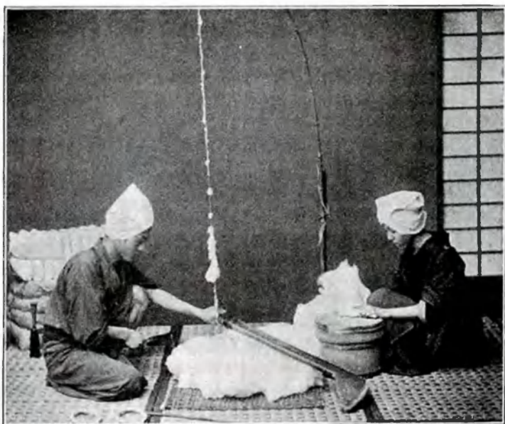
Fig 67.—Japanese form of bow used in the home for spreading cotton in making wadding and cotton batting.
