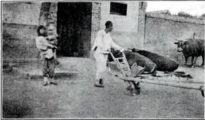
Fig. 131.—Double row seed-drill, just returning from the fields to the village home.
