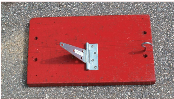
The large board with hinge and hook installed.
