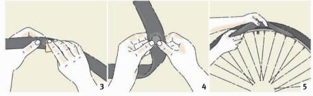
**3. Mark the hole** with chalk from your repair kit. Sand the area with sand paper, and dry the tube. **4. Apply a thin layer of glue** and wait until it starts to dry, then place a suitable patch of rubber over the puncture. Press down firmly. **5. Check the inside rim** of the tire to make sure there are no thorns or glass that will puncture it again. Fit the inner tube when it is slightly inflated.
