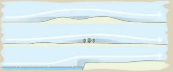
The gray areas above show where turbulence is created when the wind blows over hills (long areas of turbulence) and over a cliff, where the turbulence is relatively short.
