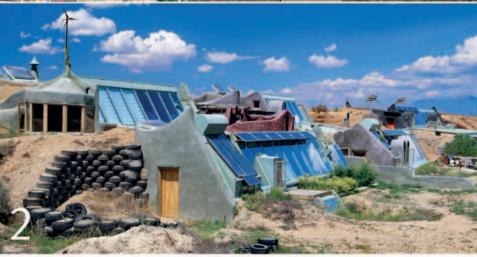
**1. The first environmentally friendly housing development** in the UK—Beddington Zero Energy Development (BedZED). Homes are made from reclaimed or natural materials. **2. Earth shelters** in New Mexico are made from rammed earth and car tires (see pages 48–49). **3. A zero-carbon house** in Kent, UK, needs no fossil fuels for heating. Its vault shape gives it high thermal mass.
