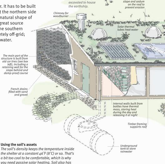
(see below). Its soil roof means you don't lose any growing space on your plot: planting your roof can even help prevent erosion.
