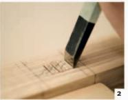
**1. Mark out** the shape of the mortise. Lay the other piece of wood across and draw on either side. Draw a second set of lines inside: the slot needs to be smaller than the width of the second piece of wood. **2. Chisel out** the mortise using a mallet. Mark out the length of the tenon and run the lines over the end of the wood using a set square.
