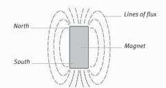
**Lines of flux** between the north and south ends of a magnet are invisible.
