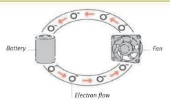
**Direct current** can be used for small appliances that are often associated with camping, such as a 12V kettle or a fan.
