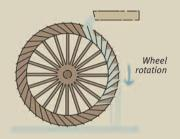
A backshot wheel is the most efficient and can convert nearly 90 percent of the water energy into useful power.
