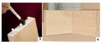
**3. Brush** dowels and joint with wood glue, and fit the dowels into the holes in the opposite piece of wood. Clamp until the glue sets. **4. The finished joint**.
