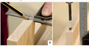
Measure and mark the center of the end of the wood with a metal ruler and a pencil.
