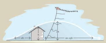
The turbulence caused by an obstacle begins twice its height before reaching the obstacle and carries on for 10–15 times the height after the obstacle, peaking at twice its height.
