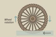
**Undershot wheels** are very inefficient (up to 20 percent) and are used when there is no head. They are basically paddles on a wheel that are driven by the water flowing under the wheel.
