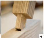
**3. Cut out** the tenon with a sharp saw. Tidy it up with a chisel. **4. Insert the tenon** into the mortise. Adjust the fit with a chisel if necessary. Add glue for extra strength.
