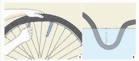
1. Remove the inner tube using levers. Then pump it up and listen for any hissing noise, or hold the tube near your face and rotate it until you feel the air escaping.
