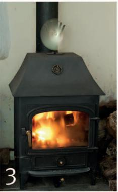
A well-designed burner is extremely efficient, preheating the air that is drawn in prior to combustion so that the flow of gases will ensure that as complete combustion as possible takes place. If you want to make one yourself, there are patterns on the internet that show how to make a wood burner or sawdust burner out of old gas cylinders.
