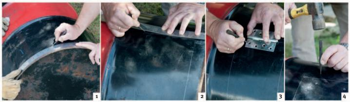
1. Mark the door of the smoker by drawing a small rectangle at the base of the drum using a metal ruler. It should be at least 6 x 10 in (15 x 25 cm). 2. Score the shape using a metal scribe. 3. Mark the position of the holes for the hinges on one side of the door using the scribe. 4. Dent the hinge holes with a punch to stop the drill from sliding around on the metal.
