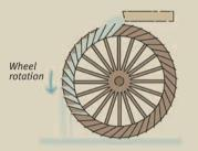
**Overshot wheels** can achieve up to about 70 percent efficiency when converting water energy into power.
