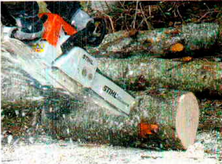
Notching the logs
