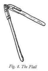
elbow height when stood on the ground. The links are of willow, the length of an extended finger, and are joined with a strap. The arm is of cherry, the length of a man's arm and extended fingers.
