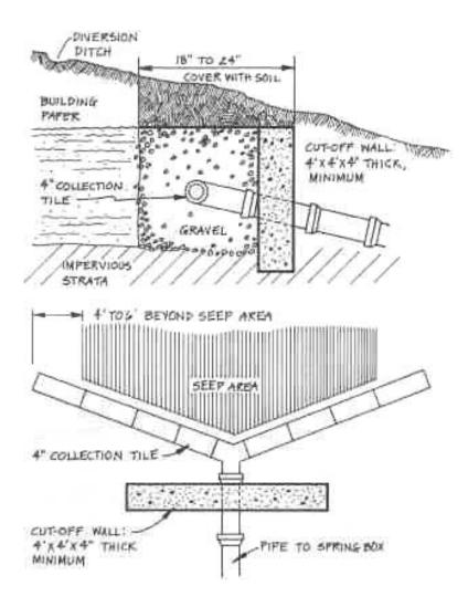
Sometimes, especially in low places, you can just dig out the spring and build a spring box over it or right adjacent to it. In one situation shown, a permeable rock wall allows the water through, while in another, perforated pipe collects the water.
