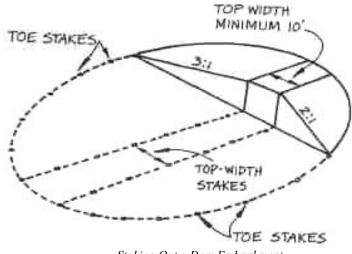
Staking Out a Dam Embankment
