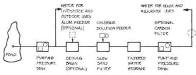
Filtering and Disinfecting Water from a Pond
