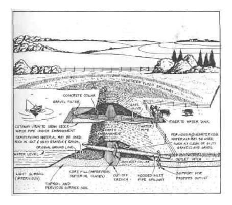
The next most important part of the picture on page 157 is the flood spillway at the upper end of the dam. This is also called an emergency spillway. Its role is to keep excess water, in times of heavy runoff, from going over the dam. Water going over the dam would quickly wash it away. The spillway is kept sodded and is built with a much more gentle grade than the dam, so water can flow harmlessly down it. Sometimes spillways wash out a little and have to be repaired.
