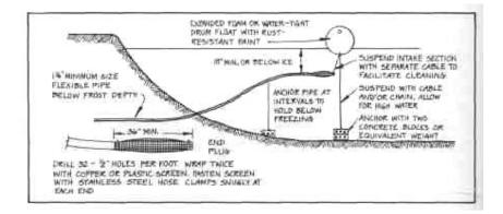
Homemade Suspended Filter Intake
