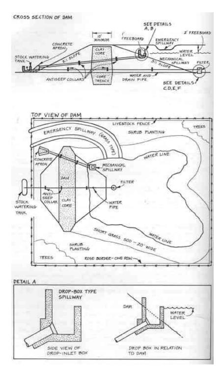
laws in your state do not require the pond to be built so it can be drained, by all means do build a drain into your pond. In most, if not all, cases, there will be times when you will want to drain the pond.
