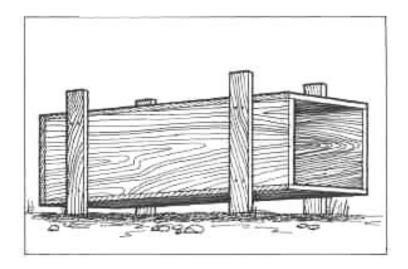
A box 1 foot square by 3 feet deep can be constructed from 1 x 12 rotresistant lumber.
