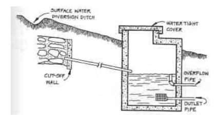
For a point spring, dig down into the ground along the line of flow until you find a place where water is at least 3 feet below the soil surface, engineers advise. Install a cut-off wall of concrete or plastic, inserting a pipe through the wall to draw the water out into a spring box. Be sure the pipe is slanted well downgrade from the cut-off wall, so pressure doesn't build up against spring flow.
