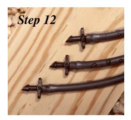
**Step 12.** You will need two drippers/emitters per bucket to insure even irrigation. Cut the drip lines from 1/4" tubing being careful to leave plenty of extra length for ease of use and maintenance. Drip lines are connected to the feed manifold using .16" barbed joiners as shown here.
