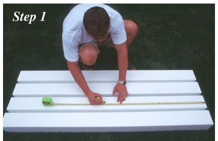
Step 1. Using either the template provided or your own design, you must first layout each of the holes to be cut. It is best to mark and measure them center to center. Make sure to pay close attention to avoid any mistakes which can be very costly in both time and materials.
