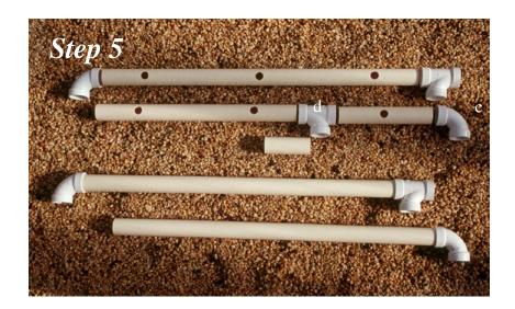
Step 5. Layout the drain and top rails that have been cut and drilled according to the parts list. Here, the two uppermost pipes make up the 6' drain rail. To prevent returned nutrient from filling the stands, you need to plug up the two 'L' fittings on either end and the single 'T' fitting that holds the two sections together in the middle of the 6' span (labeled a,b,c.) The drain spout (d.) should remain free and clear.
