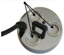
A triple transducer module with teflon-coated discs is required to generate the correct droplet size and volume of fog. The coated tranducer discs help facilitate easy removal of mineral buildup - The module shown below is nestled in a float that keeps it at the correct operating depth.
