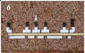
**Step 7.** Assemble the internal spray lines from the parts shown here - 3/4" FGH swivel adapter with a compression end, .375 ID poly spray line, 10 mm insert plug and a 1" rubber grommet to seal the entry point of the spray line into the growth chamber.
