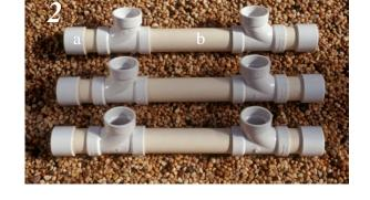
**Step 1.** Cut pieces for the 'toes'-(a) and 'feet'-(b) from your 1 1/2" PVC pipe according to the measurements given on parts list. Line up pieces as shown and test fit for accuracy before gluing.
