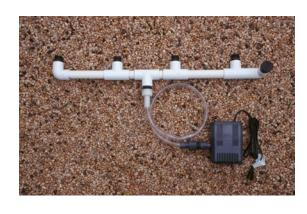
Note. Once you insert the spray lines into the compression end of the adapters, they are nearly impossible to remove without damage. Test fit everything first! You only need to insert about 1/2" into the compression end for a good seal.
