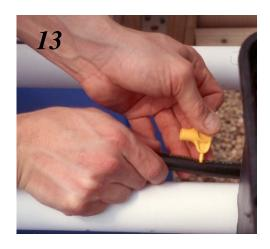
**Step 14.** Emitters are easily connected to the drip lines and inserted into your growing media. Most emitters are adjustable - space them evenly to promote even distribution of nutrient solution across the media surface and root mass below.
