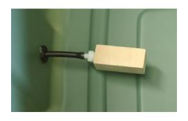
**Step 6.** Drill a 3/8" hole in the bottom wall of your container and insert the 1/4" rubber compression grommet. Pass your air tubing through the grommet and attach to your air stone.
