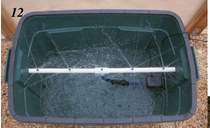
**Step 12.** Fill 'er up with water and take it for a test ride. Adjust the rotation of your spray bars so the spray is as flat as possible. Never run your Aerospring dry - the top of the pump is the lowest level you should ever allow your nutrient to reach, any lower can cause pump failure.
