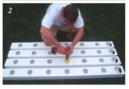
Step 2. Using the 2 7/8" hole saw and a cordless drill to cut each of the grow sites and a 4" hole saw for the access ports (one per chamber, on right side of the chambers shown here) The 14v cordless drill I used here has cut hundreds of holes over the last year! A single charge was enough to finish the four chambers shown here each with 6 grow sites and 1 access port.
