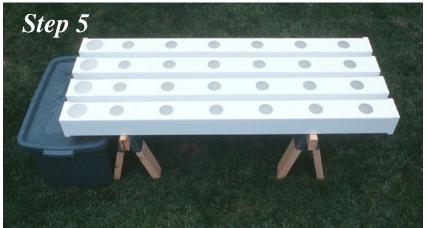
Step 5. Assemble your system so that each chamber is evenly spaced apart on the saw horse support. It is best to leave yourself a few inches of space between the bottom of the chambers and the lid of your reservoir. Measure the spacing from the center of one chamber to the center of the next to determine the spacing of spray lines on the manifold below.
