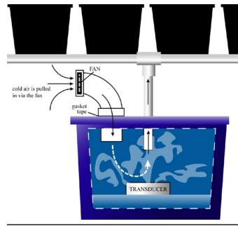
Fig. 1. The concept and operation is quite simple. An external fan forces fresh air into the reservoir where it mixes with the fog created by the transducer. Since this mixture can only escape through the drain manifold, it ends up filling the Dutch Buckets through their drain fittings. Excess solution that collects in the buckets drains back into the reservoir in the same tubing with no impedance to the fog.
