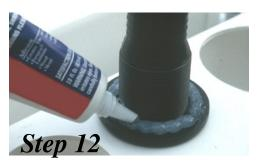
**Step 12.** If you choose to use the bulkhead fitting, be sure to seal with Aquarium-safe silicone sealant to prevent leaks. Apply as shown here. If you choose to go with the grommet method, it helps to apply a thin coating of nontoxic silicone grease to the inside of the grommet to allow the level tube to move up and down easily.
