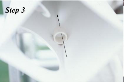
Cut 3/4" - 1" sections of 1/2" PVC pipe to make the spray line clips shown above. They are glued into the chambers using PVC cement. For best results, use PVC primer before applying glue to soften the material and provide a better glue joint.
