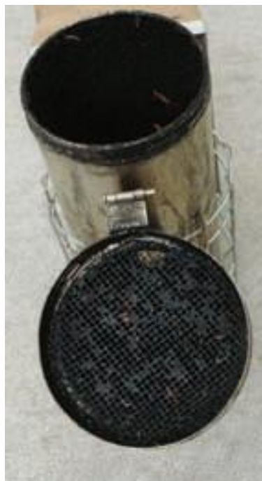
This simple #8-mesh-wire screen filter prevents the blowout of fuel particles and sparks that could start a fire.
