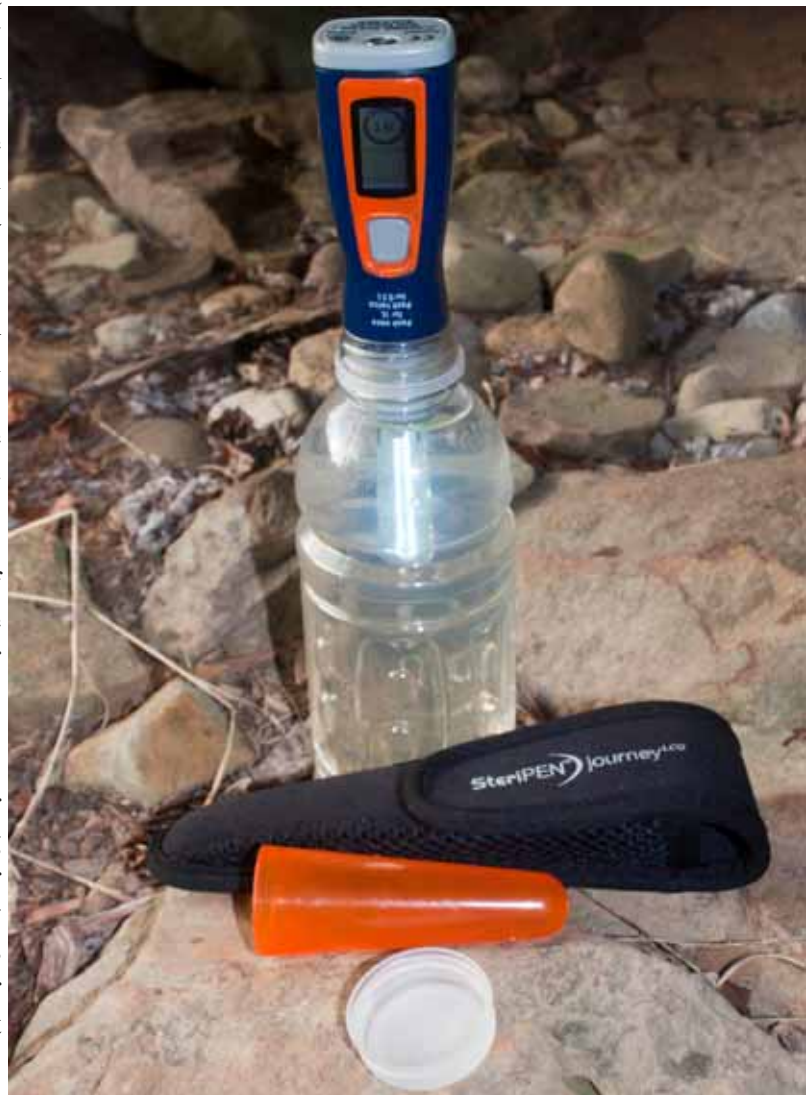
Here we see the SteriPEN in the most common setup for usage. Any container which will allow the contacts to be submersed may be used. 1 Liter maximum.
