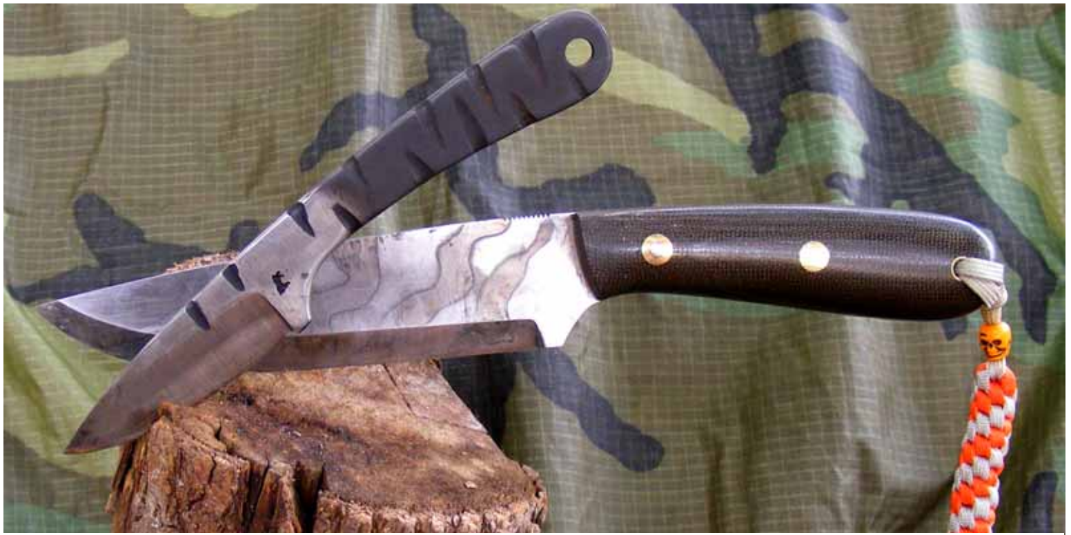
The Author's preferred carry for woods time is the Pathfinder knife from BHK, along with the Large Tiger Knapp from the same. The tiger Knapp is great at detail work, cleaning small game, and small camp chores, and the Pathfinder with its carbon steel, scandi grind blade makes quick work of wood, and larger game.
