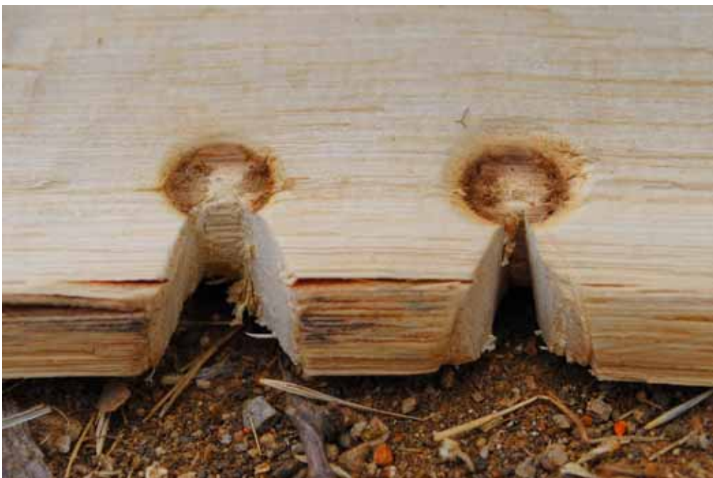
The image above shows an improper notch on the left with a proper notch on the right.
