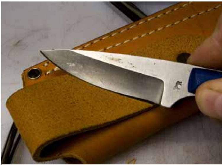
Figure 4: The beltloop is another area that can be used as a strop.
