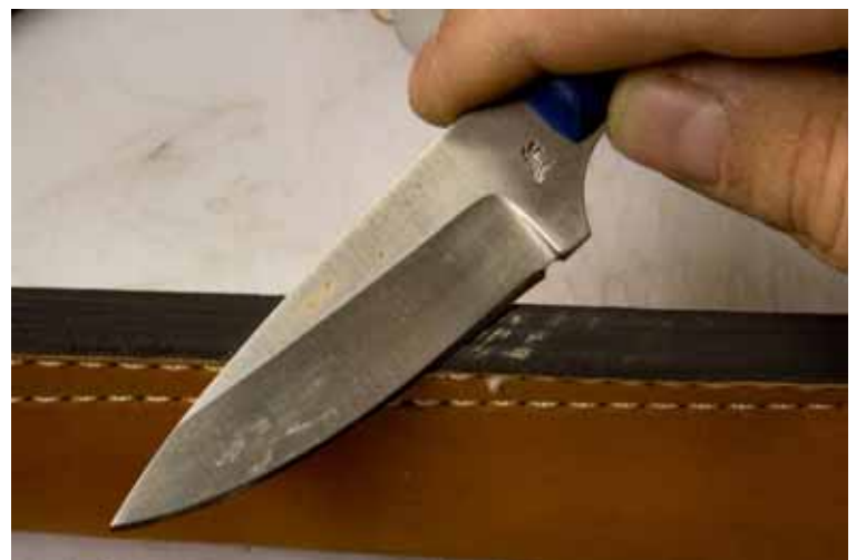
Figure 3: Using the edge as a strop to bring back the hair popping sharpness.
