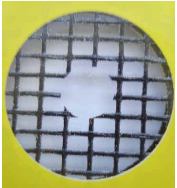
Photo 1 (left) shows the retro-reflective grid in a Vector 1 acrylic cased signal mirror, which does not have a hole in the grid. Photo 2 (right) shows the retro-reflective grid in an AMK Rescue Flash signal mirror which does have a hole in the grid. The hole does not affect the retro-reflectivity of the mirror, it is just a different design.
