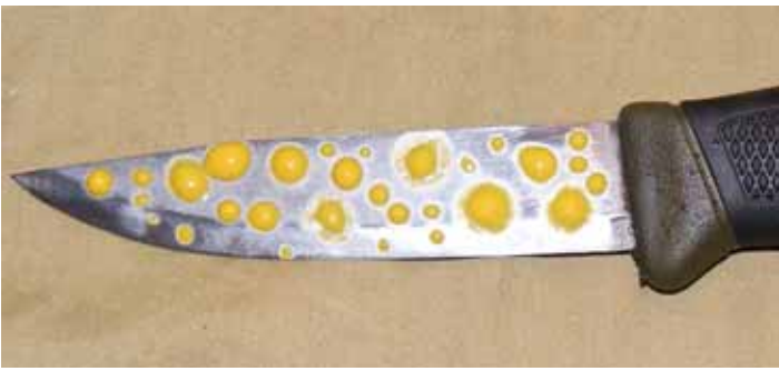
Mustard applied in rain-drop pattern using a toothpick to dip and just lightly touch the blade.
