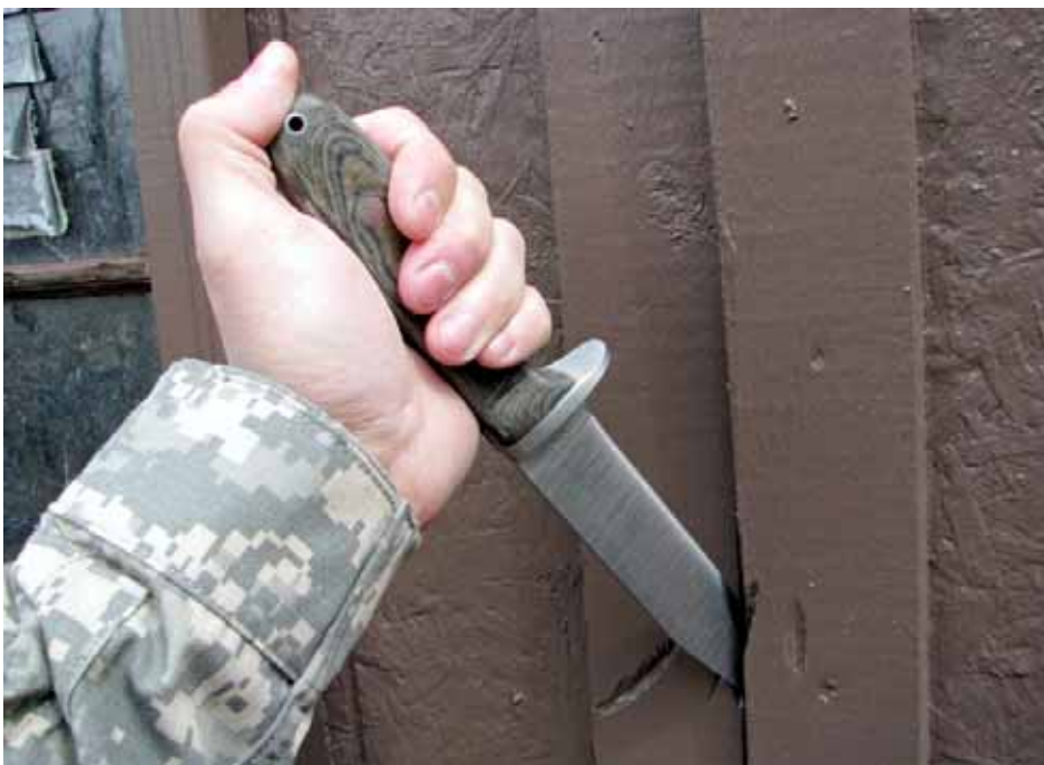
While prying isn't the intended use of the knife, during testing the blade was bent during batoning and returned to true. Gossman's heat treat creates a strong blade.
