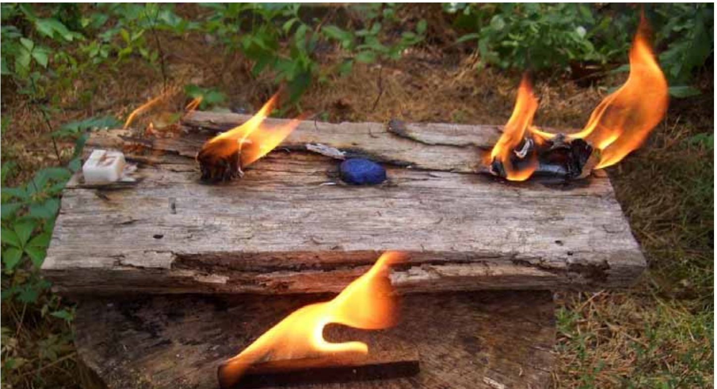
The burn after 1:30 min/sec. The cotton ball is second from left and the Pitch Witch is to the extreme right. The Esbit is still maintaining its original shape at left, the Trioxane is burning with an almost invisible flame (center) and the obvious Coughlan's stick in the foreground. All are burning well.
