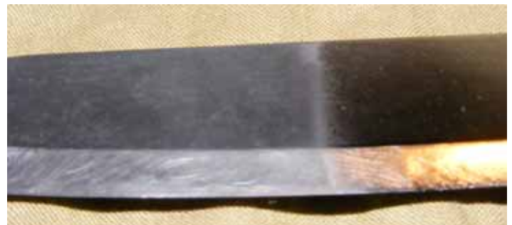
Above: After one hour soaking in apple cider vinegar with half of blade cleaned to show difference.
