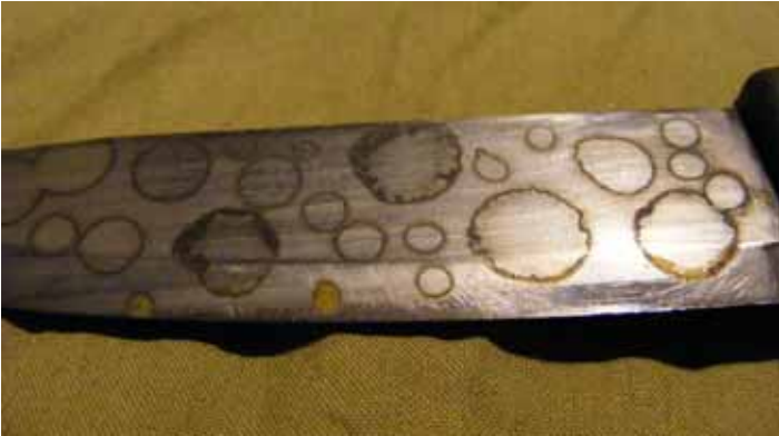
Results after letting mustard set for 30 minutes...a longer soak time will result in a blacker, and deeper etched finish.
