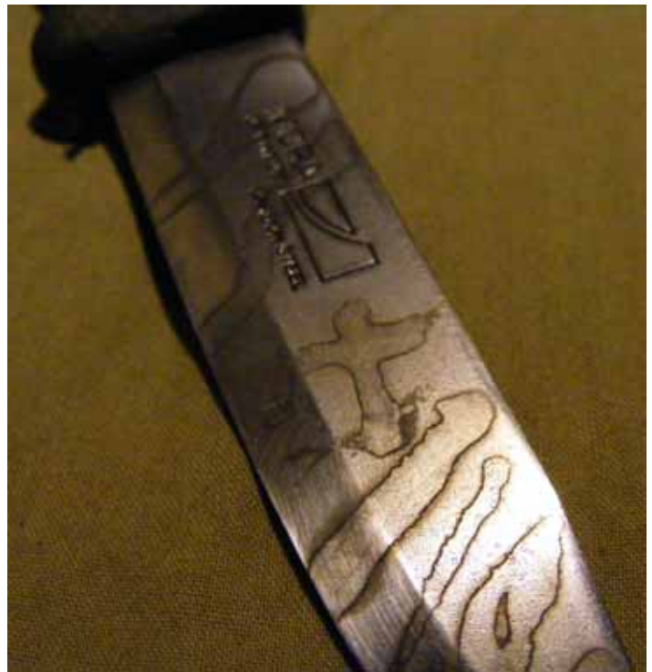
Results from striping. Again, a longer soak time will yield a deeper etch. This was 30 minutes.
