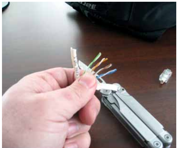
The same Network Cable with the connector removed exposing wire within.
