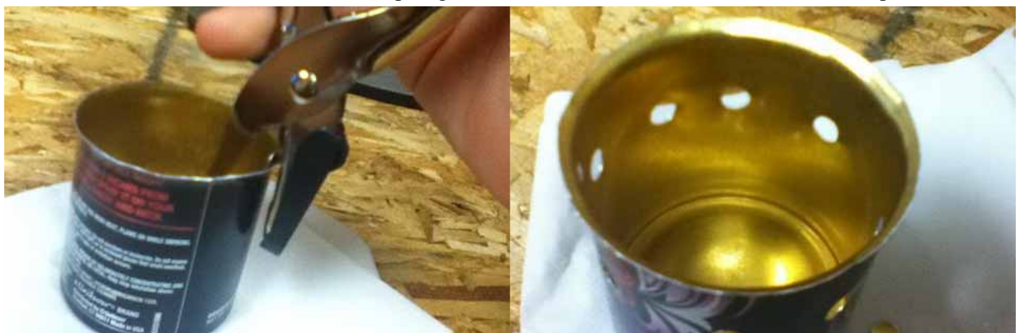
Photo 5: Punching lower burn holes
