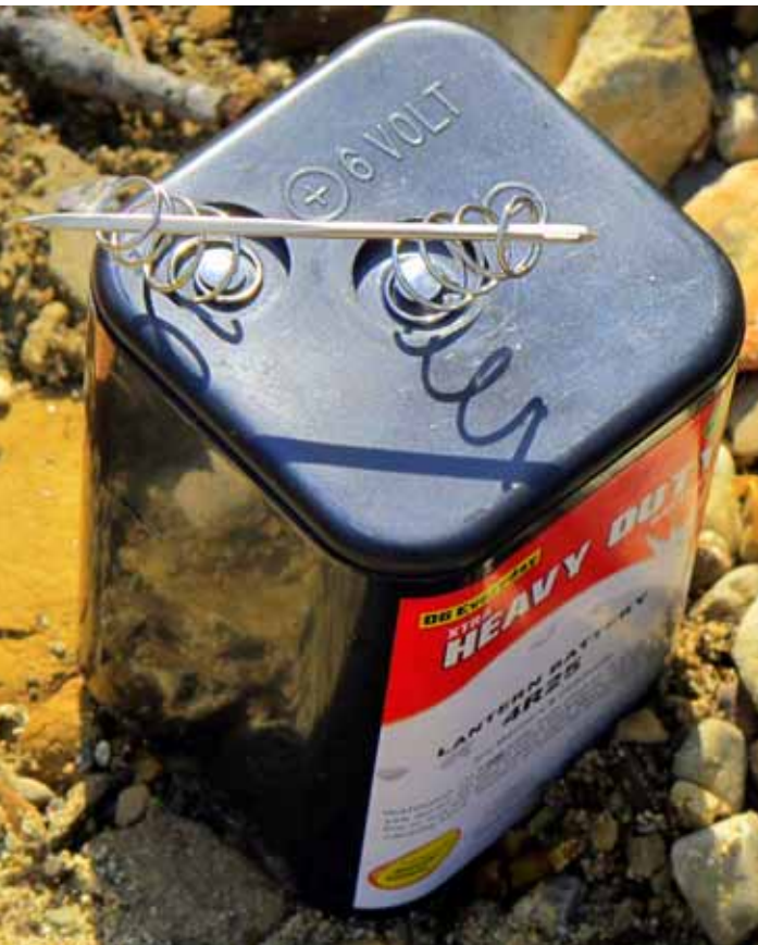
Magnetizing your needle electrically or by contact will enable it to be used as an emergency directional device as well.
