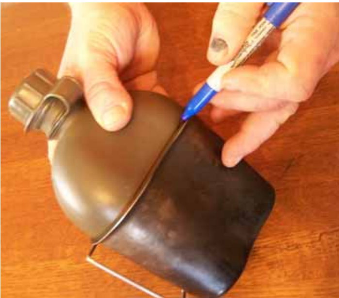
Marking the canteen to cut
