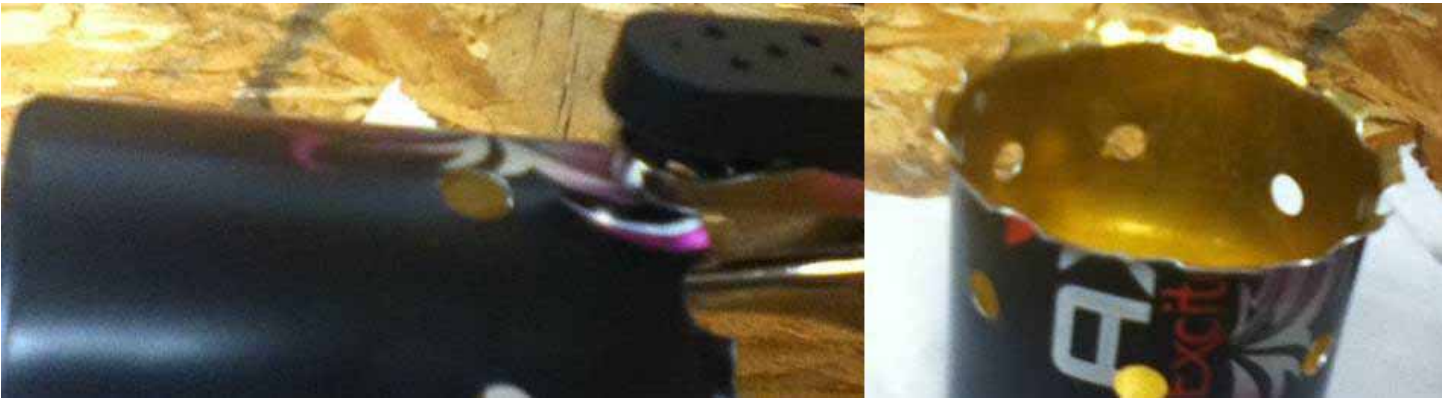
Photo 6: Punching upper vent holes
