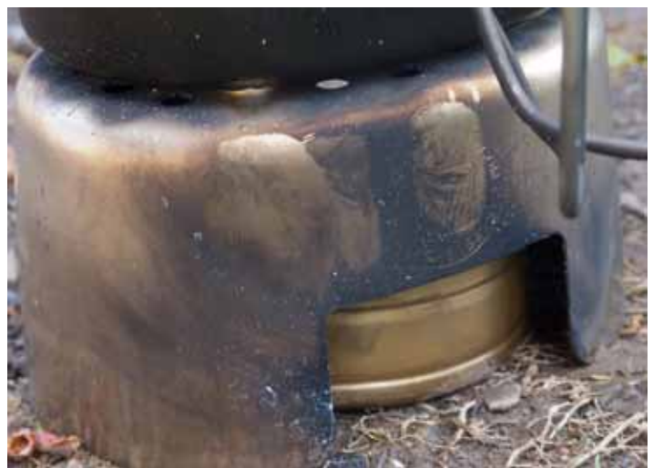
The GrillTop allowed a Trangia stove with simmer ring to fit underneath and proved to act as an efficient wind screen when the stove was in use.
