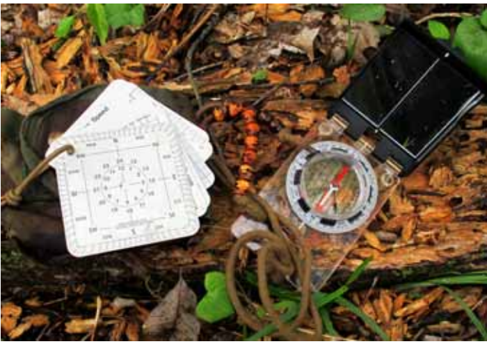
A Good compass with a sighting mirror and bezel ring will give you many benefits from navigation by visual bearing to signaling for rescue.
