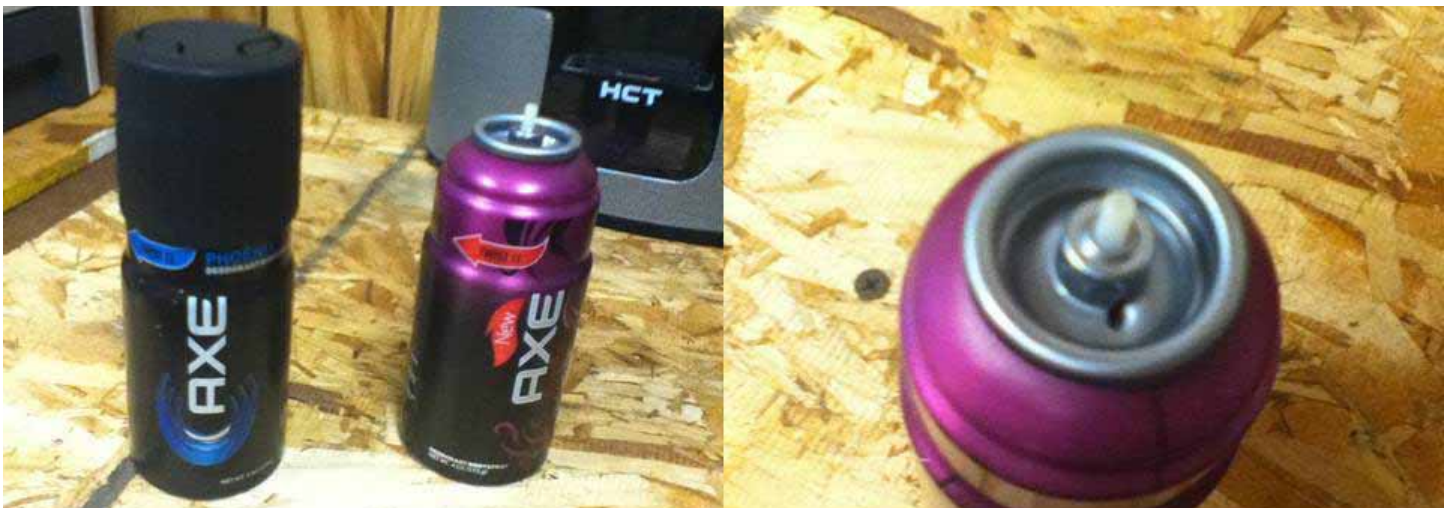
Photo3: New Axe can and can to be used, can with nail hole to depressurize.
