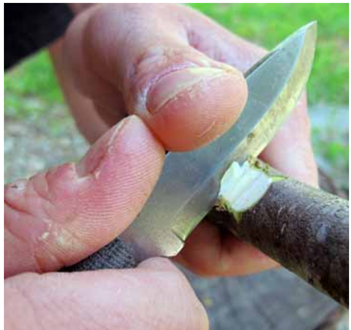
But using both thumbs, a lot of pressure can be exerted behind the blade to carve a notch.
