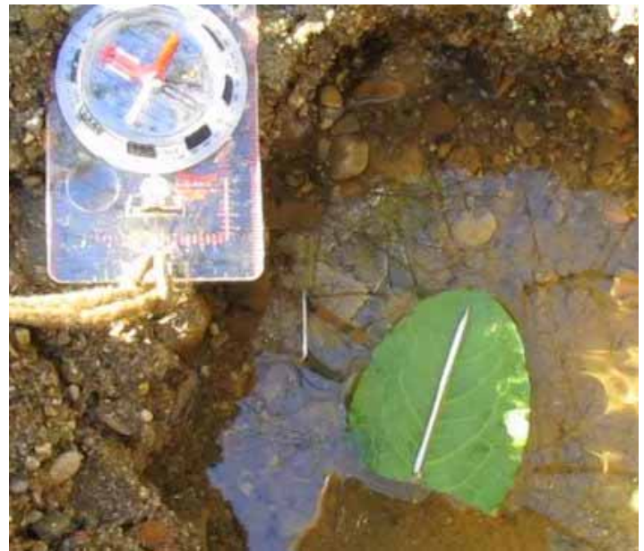
A Magnetized canvas needle being used as an impromptu compass.
