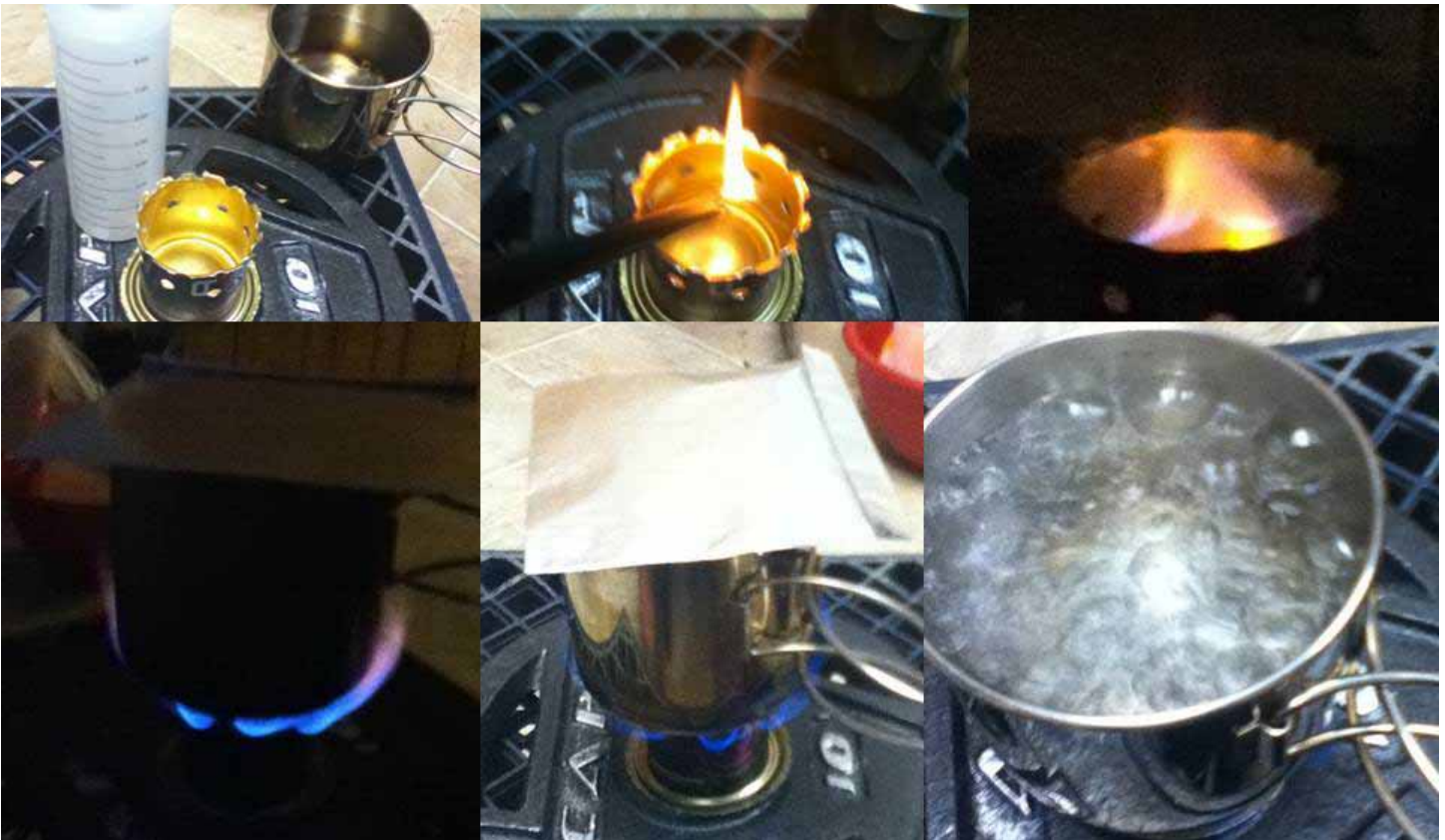
Photo 7: Completed stove and its inaugural burn, boiling in less than 6 minutes with water from the refrigerator.
