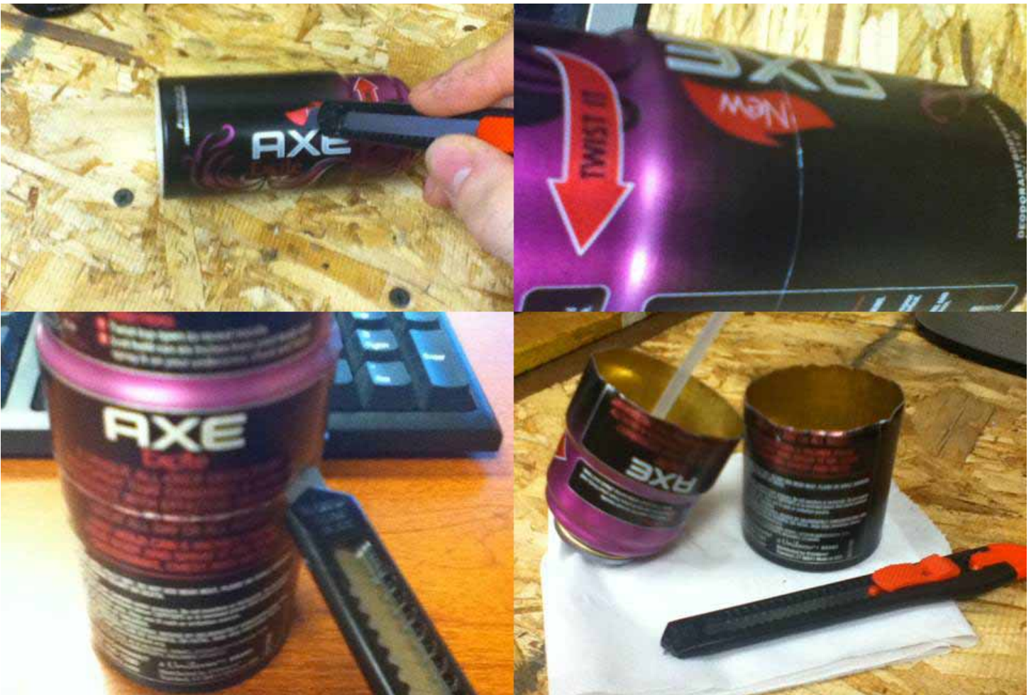
Photo 4: Marking, scoring, cutting and separating the can halves
