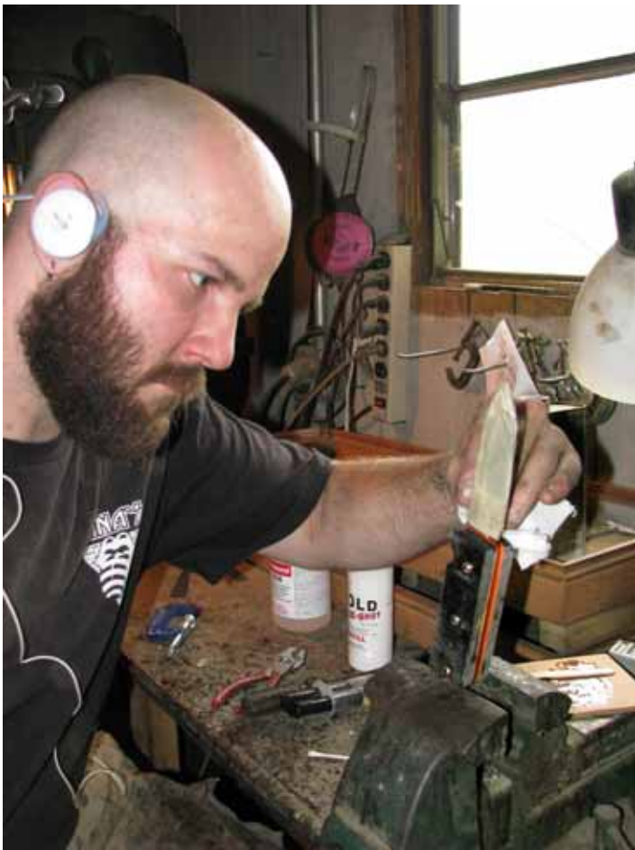
Matt gluing a black bushcrafter with orange liners.
