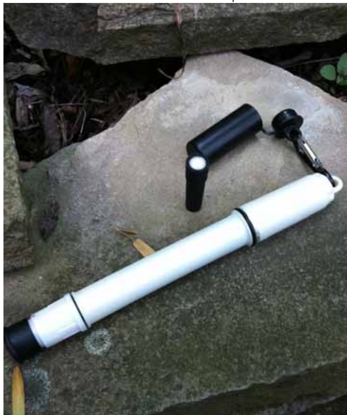
Above: The pre-filter is ready for use for the really dirty water.
