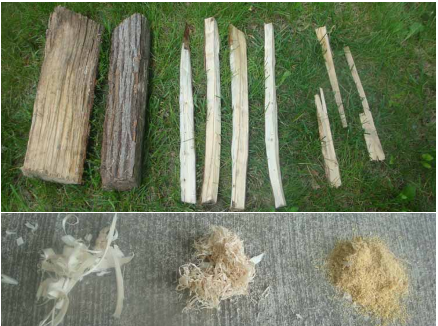
Figure 2: Two photos to illustrate wood being broken down to show increasing surface area. (Photos by the author)
