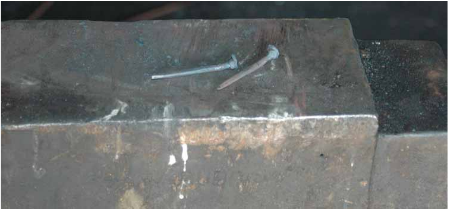
Finished, hand-forged nails.
