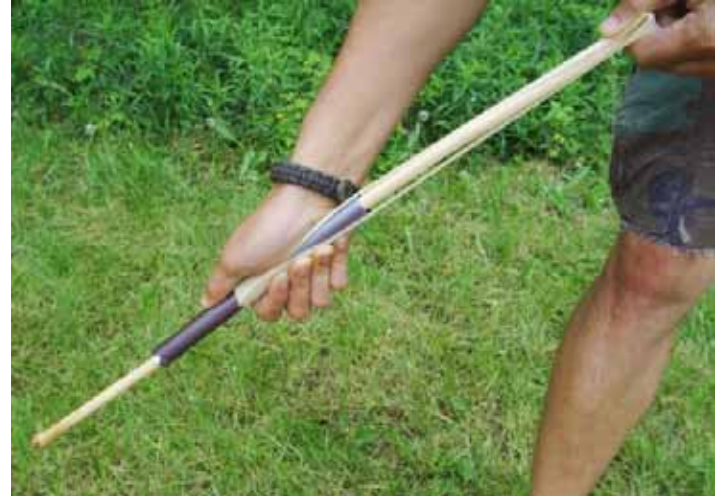
Here the author demonstrates how to hold the Paray dart shooter to eliminate the need for cordage attaching the elastic to the pipe.
