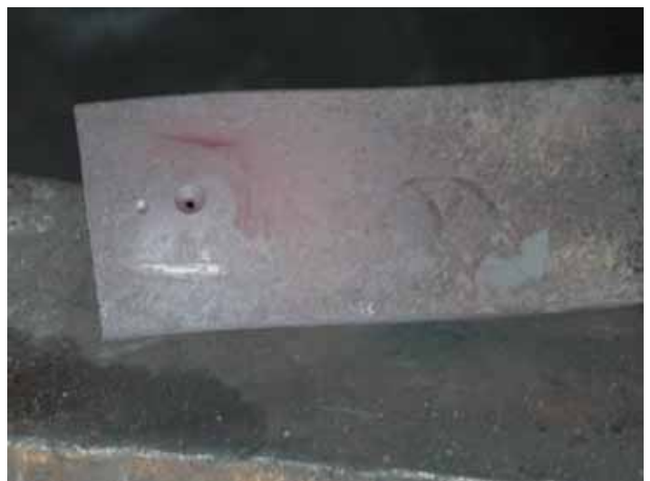
Top Right: The hole has been drilled in the leaf spring and is ready for "sinking".
