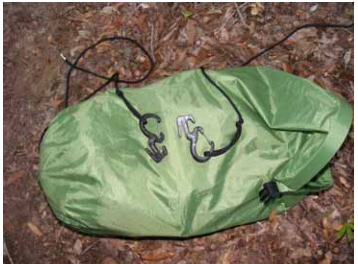
A small set of figure 9's with a short length of cordage makes for a fast hang of the tarp, should the weather turn south.
