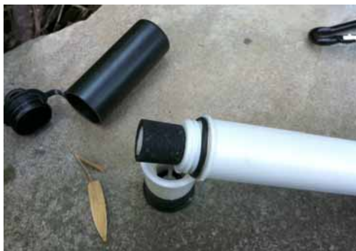
The Pre-filter installed.
