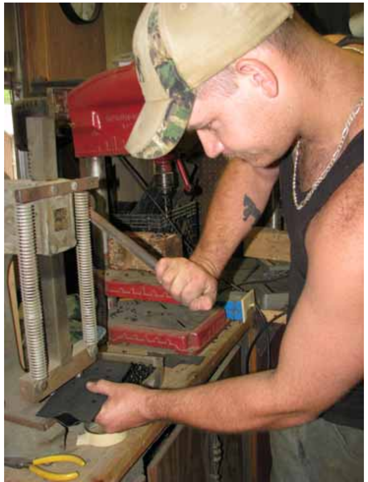
John putting rivets in the PLSK kydex sheaths.
