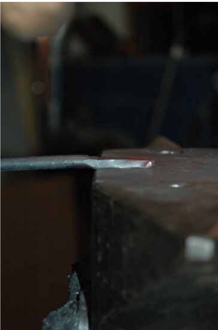
Left: Building the shoulders of the nail.
