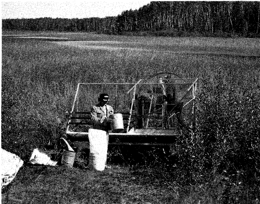
Figure 46 At least two people are required to harvest wild rice efficiently. As soon as the engine is stopped the speedhead can be unloaded, any leaves and stems removed, and the wild rice bagged, weighed, and labelled.
