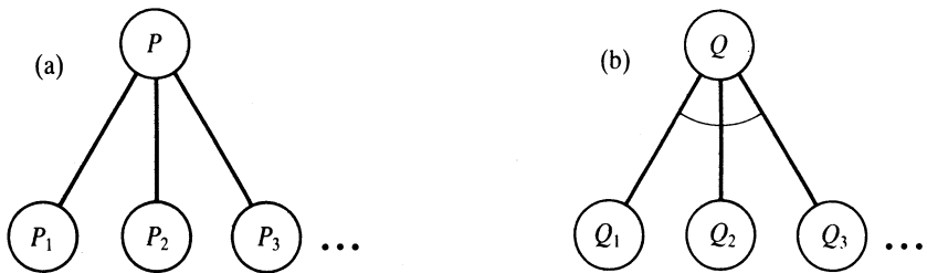
Figure 13.3 (a) To solve P solve any of P_1 or P_2 or... (b) To solve Q solve all Q_1 and Q_2 ...
