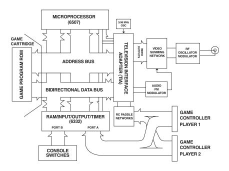
**2.2** This high-level sketch of the components of the Atari VCS and how they are put together, called a "block diagram," is based on a hand-drawn one shown by Decuir in his presentation "Three Generations of Game Machine Architecture."
