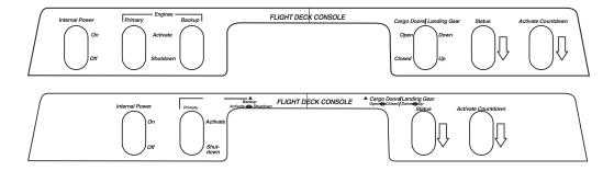
**6.3** These paper overlays for *Space Shuttle* are intended to be placed on the Atari VCS console itself. They have cutouts for the VCS switches. Both of these overlays were provided with the cartridge so that the game could be played with either a six-switch console or a four-switch console. The creases in the center of the overlays are from where they were folded to fit in the box.
