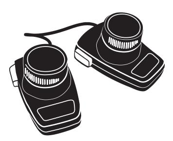
**2.1** The Atari VCS paddle controllers work by measuring output from an internal potentiometer. Atari also released a driving controller for use with  $Indy\ 500$ . It has almost the same appearance, but its knob rotates freely, rather than stopping at the extreme left and right.
