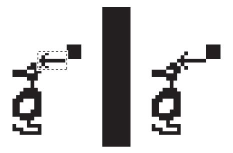
**3.2** If *Adventure* had used bounding box collision detection, as on the left, this arrangement of sword and dragon would indicate a collision, because the box enclosing the former intersects the latter. Because the VCS hardware implements collision detection by overlapping bits, as on the right, there is actually no collision in this situation.
