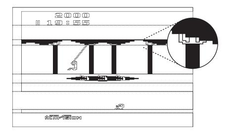
**6.2** The distinct horizontal sections of a *Pitfall!* screen from the programmer's perspective. *Pitfall!* uses the TIA's graphics registers in ways that were not originally intended, as many games did around this time. In this image, areas drawn with playfield graphics are shaded in black. The branch details between the trunk and canopy are drawn with sprite graphics, as can be seen more easily in the inset detail.
