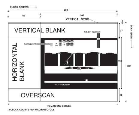
**2.4** The Atari VCS television image is broken down and key regions and measures are indicated. This television protocol image is based on the one in Wright, *Stella Programmer's Guide*.
