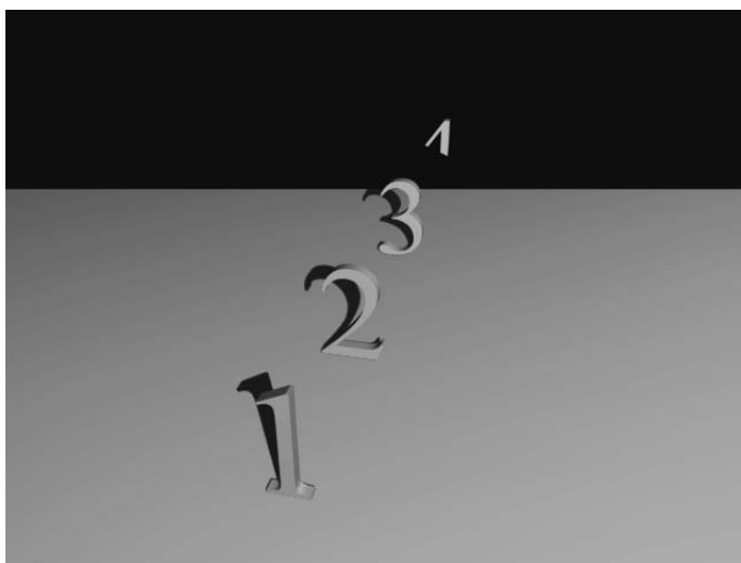
Figure 11.15 A far clipping plane cuts off the distant extents of a scene.
