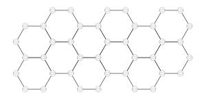
This is a single plane of graphite. A piece of graphite consists of many of these planes layered in a stack. (The chemical bonds between the planes are much weaker than the bonds inside the planes, which explains why graphite writes it can be sheared so that the planes slide off and are left on the paper.) A convienent unit of length can be made by decomposing the hexagonal ring into three regions that are rotations of this *unit cell*.
