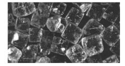
Remarkably, the explanation for the cubical external shape is the simplest one possible: the internal shape, the way the atoms lie, is also cubical. The internal structure is pictured below. Salt is sodium cloride, and the small spheres shown are sodium while the big ones are cloride. (To simplify the view, only the sodiums and clorides on the front, top, and right are shown.)
