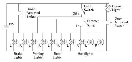
The designer of such a network needs to answer questions like: How much electricity flows when both the hi-beam headlights and the brake lights are on? Below, we will use linear systems to analyze simpler versions of electrical networks.
