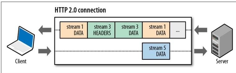
Figure 1-3. HTTP/2 request and response multiplexing within a shared connection
