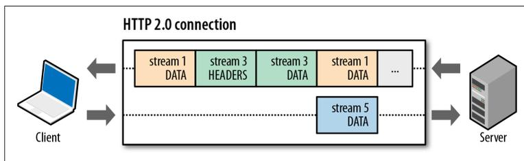
*Figure 1-10. HTTP/2 request and response multiplexing within a shared connection*
