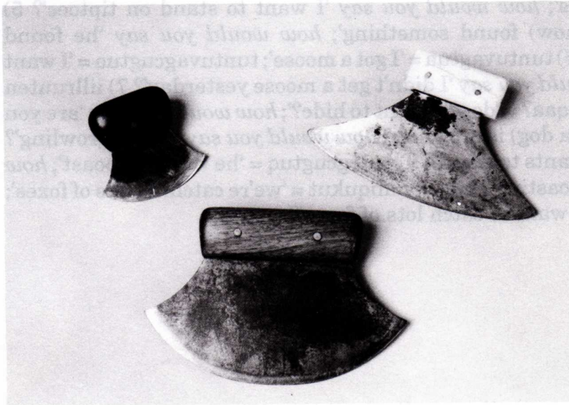
Uluat are made from old saw blades. In olden times they were made of stone with handles of wood, bone, antler, or ivory. Photo by Richard Veazey.
