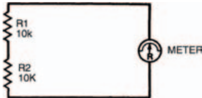
Figure 2.5 A circuit diagram of two resistors in series. The meter is represented by a round symbol
