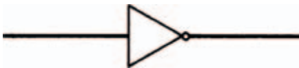
Figure 10.4 The symbol of an inverter — the simplest form of digital logic gate
