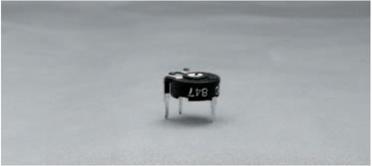
Photo 6.1 A horizontal preset resistor
