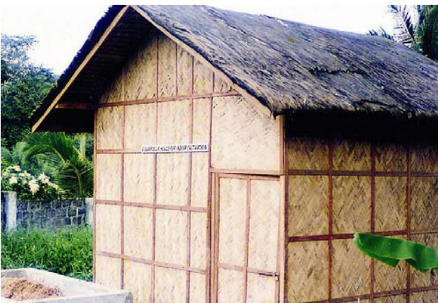
Figure 19. Mushroom house made up of bamboos, sawali, and nipa roof
