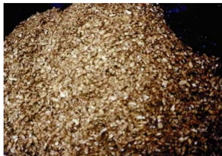
Figure 5. Deeper color of groundnut shell after soaking
