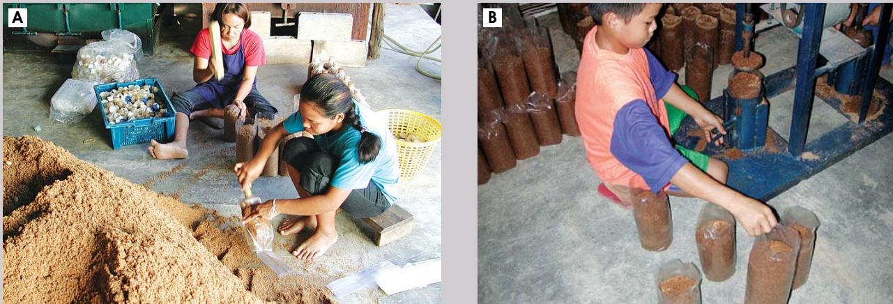
Figure 5. Bag filling and compacting A: Manual filling and compacting with rod B: Compacting bags with machine
