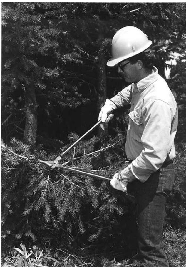
Lopping shears allow branches to be cut cleanly and flush with tree trunks.
