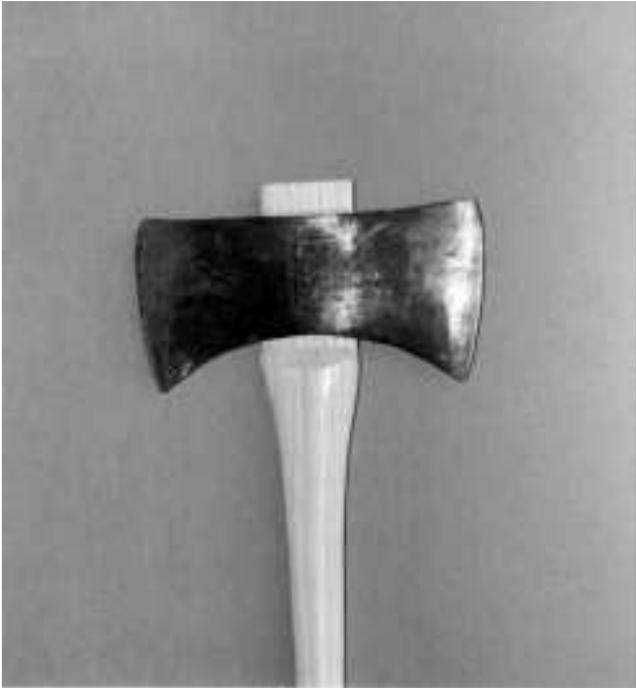
**A**—Size up the tool head and match it to the handle. Note that the handle protrudes excessively long through the head. Scribe it to be cut off.
