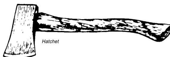
Use and maintain hatchets like regular axes. Remember that these tools are not designed for excessive pounding. Additional hazards may also exist for users because hatchets are single-grip tools.
