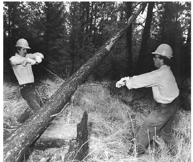
The hand chain saw performs equally as well as a conventional crosscut saw.
