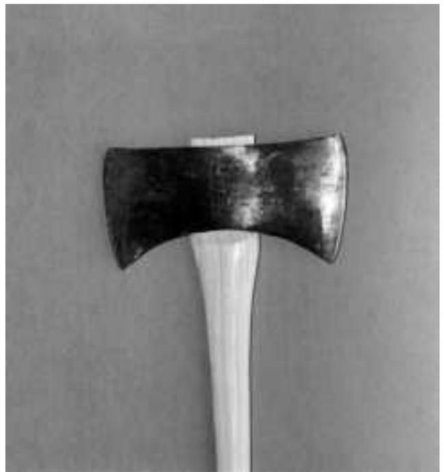
**D**—The tool head has been snug-fitted to the square seating shoulder. Note that there is about  $\frac{1}{2}$  inch excess handle above the head.
