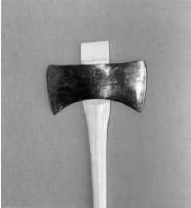
**E**—All surfaces just below the handle should be sanded smooth before the head is placed to insert the wedge. The wedge has been started in kerf.
