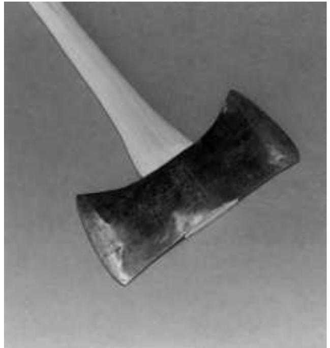
**H**—The finished mounted tool. The handle can be finish-sanded and oiled with raw linseed oil to protect against moisture.
