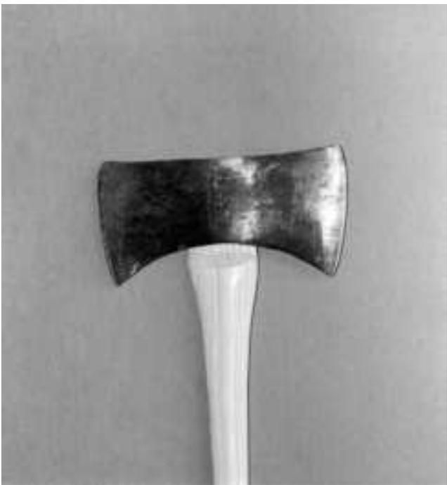
**B**—Saw the handle to about the correct length. The handle has been roughly fitted so the head slides to within about  $\frac{1}{2}$  inch of the final seating position.
