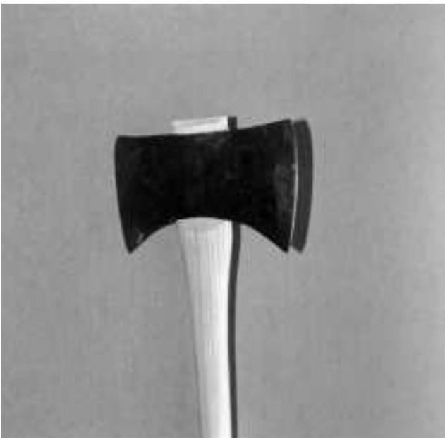
**F**—The wedge has been driven home with the alternate driving of the wedge and the end of the tool handle.
