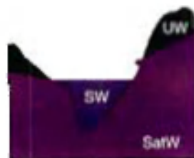
Figure 6.21 Some water may be drawn from the saturated layer and return to the surface water flow
