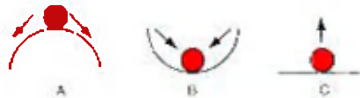
Figure 3.6 Three types of equilibrium: A, unstable; B, stable; C, neutral
