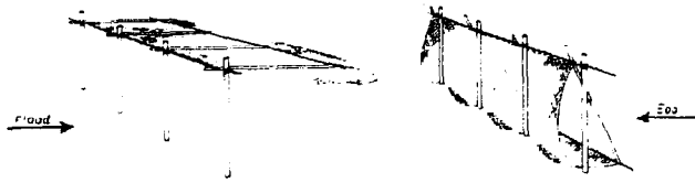
Fig 261 English 'balk net' which operates automatically during flood and ebb tide. It swings up to let the fish in and then down as the tide flows out. (Davis, 1958).
