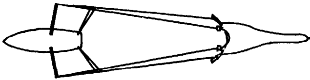
Fig 511 One-boat midwater trawl with four otter boards, used in the Belgian and Dutch fishery.
