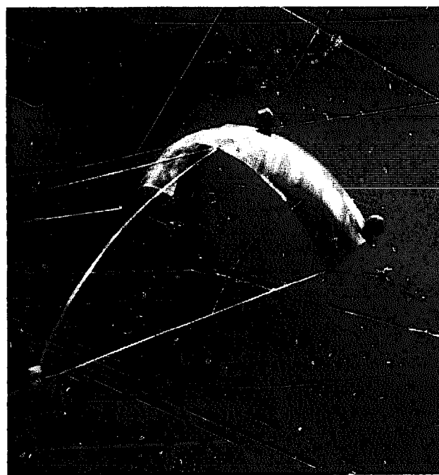
Fig 486 Sailkite for a rope trawl. (Photo: W Horn, 1980).
