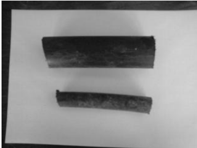
Class 3 black irrigation hose 40mm and 20mm
