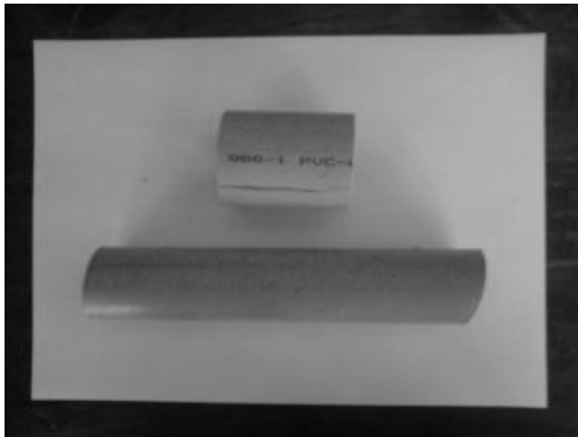
Blue PVC pipe 40mm and 50mm – suction line pumps
