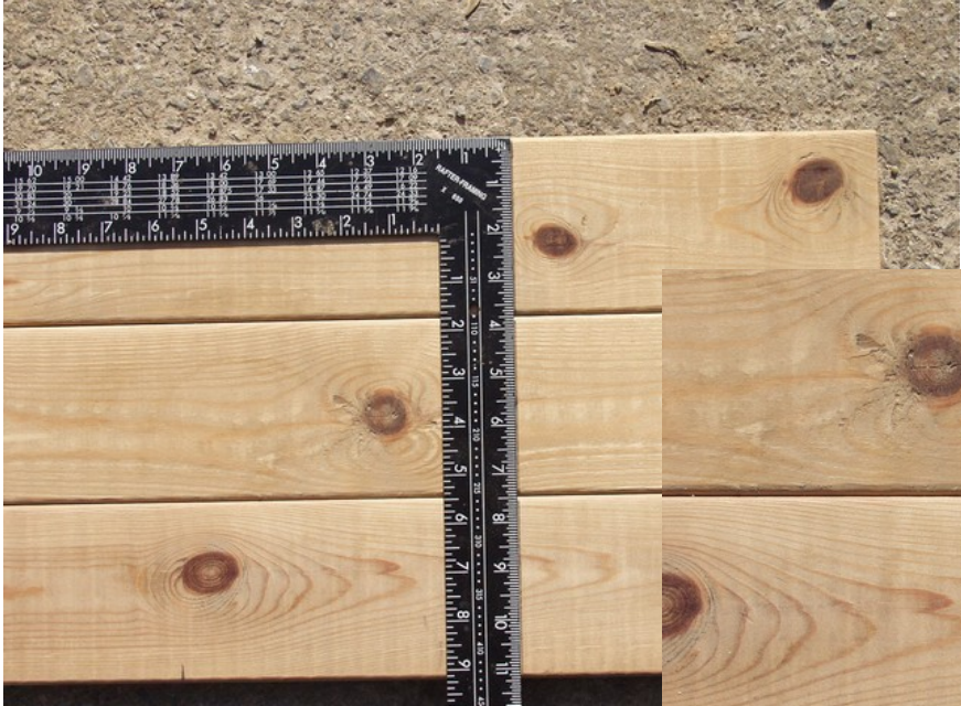
Draw a centre line to the bottom edge
