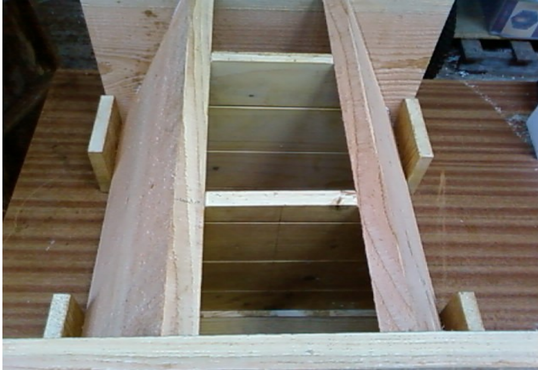
Showing the use of the jig to keep the sides in position.
