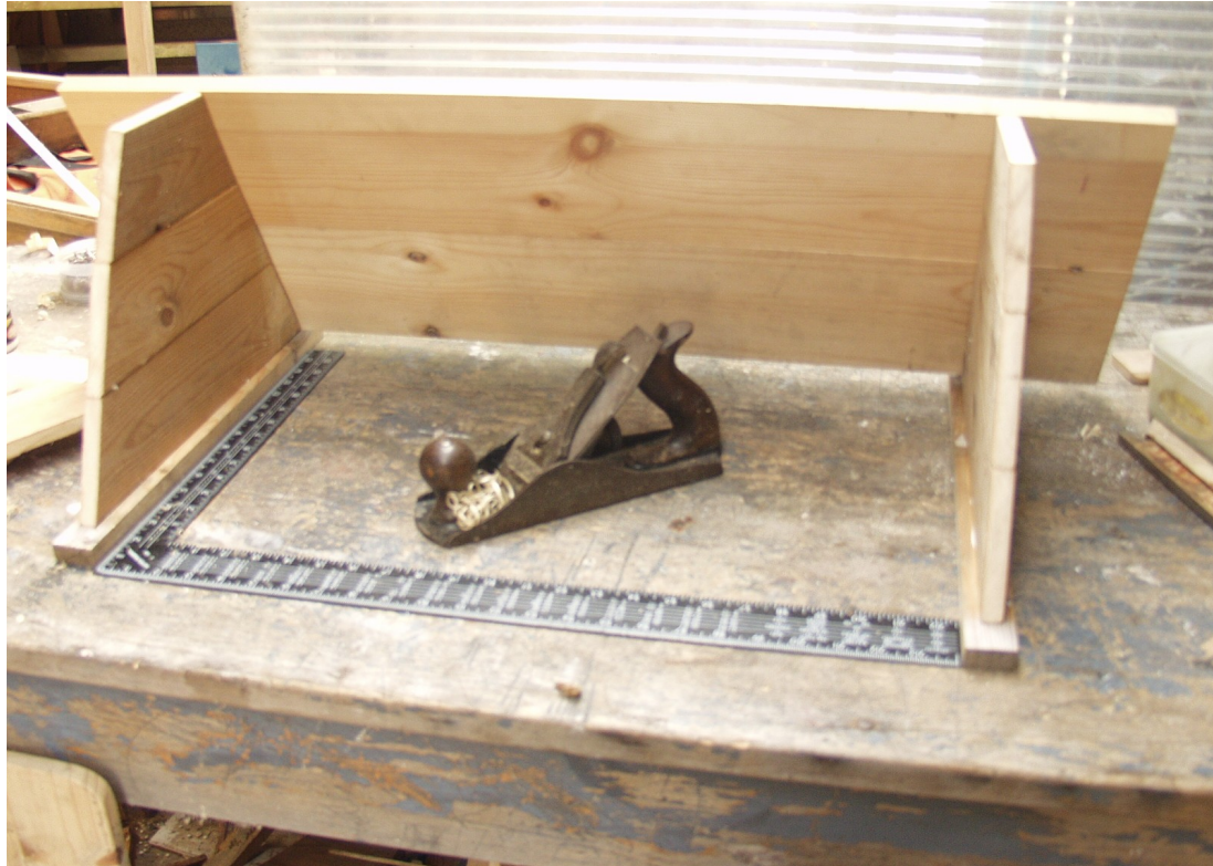
Position one of the side panels against the follower boards, resting on the top bars.
