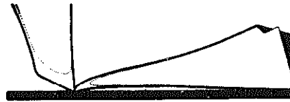
Fig. 4-10. Heavy lines show proper shape of sharp points for good penetration. Dotted lines show how worn points look before sharpening.
