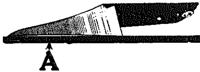
Fig. 4-11. Illustrating underpoint suction in landside of a plow share
