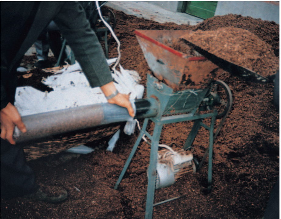
Auger bag filler commonly used in China. (Tian)
