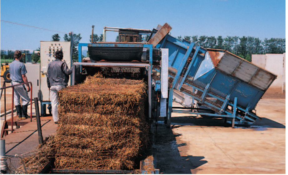
Mechanical assembly of compost materials for button mushroom ( Agaricus bisporus ) cultivation. Prewetted bales of straw are opened, and straw mixed with poultry manure and gypsum is added from the hopper on the right. Meadow Mushrooms, New Zealand. (Buchanan)
