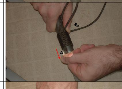
6. Trim off both ends "A" and "B" with a sharp blade and melt them closed.
