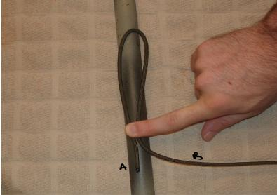
2. Take end "B" and wrap it around the object and around the mouth of the loop you have made.
