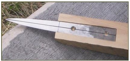
You can shape the block into a handle using these pictures as a guide after the blade is finished and ready to mount but you want this point of completion for the shaping process.
