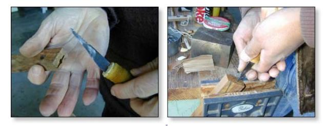
I attach the blade to the handle with 30 minute epoxy.
