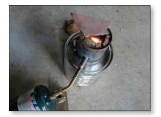
For the two abovementioned methods do the heating in a dimly lit location so you can tell when the blade has a medium red glow. This is a fairly good indication that the correct temperature has been reached.
