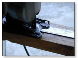
When you are deciding on the blade thickness you are going to use remember that the amount of metal that must be removed is proportional to the length of the blade times the square of the thickness. If you want a blade that is twice as thick then you have to create a pile of metal filings which is 4 times bigger. This why I like making small knives.
