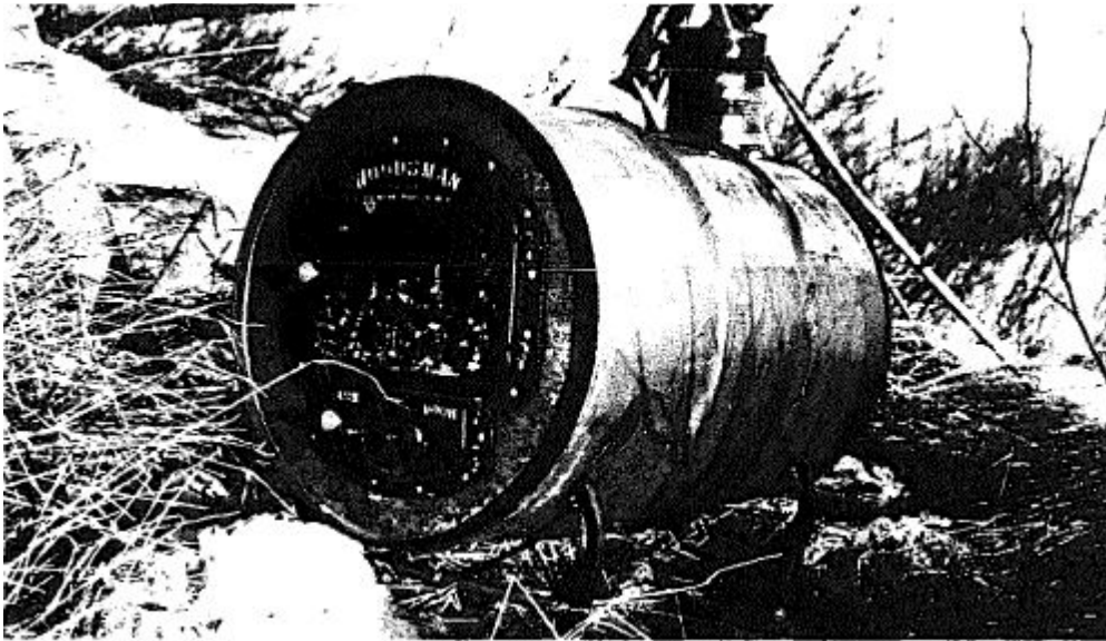
Figure 16.2 - Horizontal whole-barrel stove made with a barrel-stove kit from Fatsco. Note how a No. 10 can fits perfectly over the stovepipe collar at the rear. Made by Howard Kanther.
