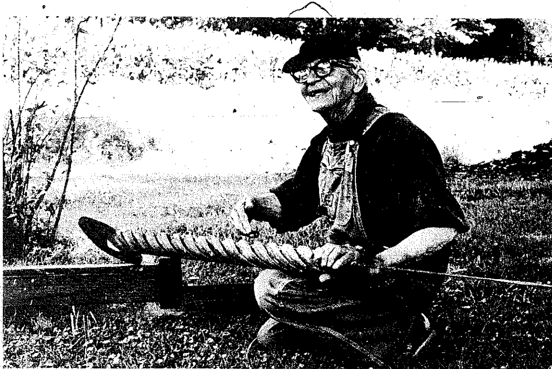
PLATE 187 Charlie Blevins with his rifling guide. The guide fits into the long wooden box in the background. At one end the box has wooden teeth that fit into the spiral grooves forcing the guide to twist as it is pushed into the barrel or drawn backward through it.
