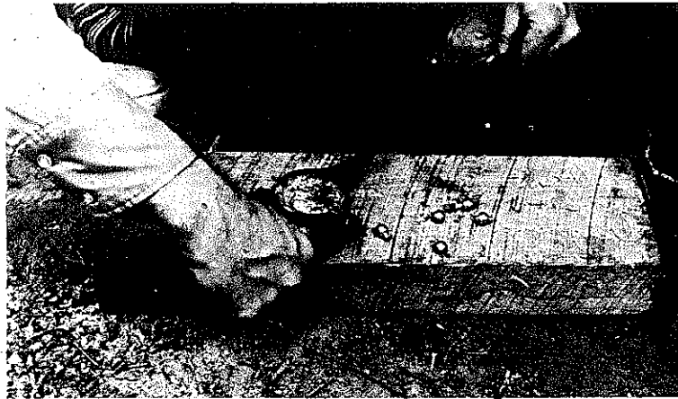
PLATE 316 Hershel pours hot lead into a mold and makes a ball. The gunsmiths call it "running bullets" or "running balls."
