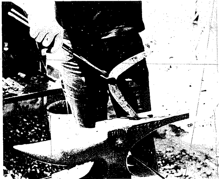
PLATE 129 Putting the bend in the toe of the horseshoe.
