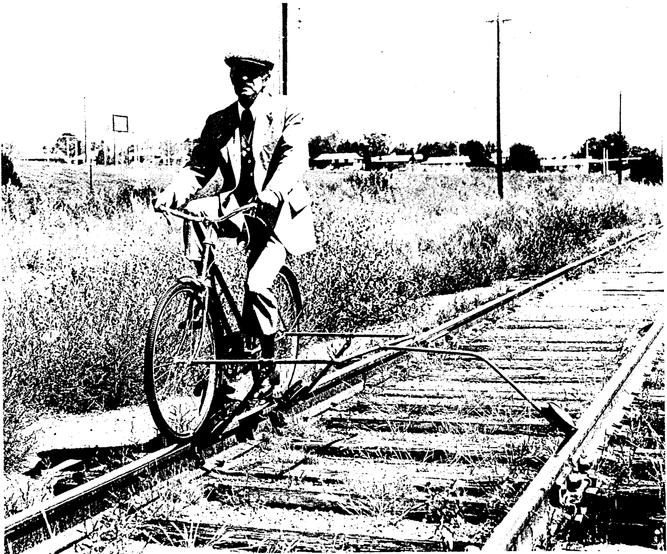
Figure 6-11 The railbike is a viable form of transportation in many sections of the world.
